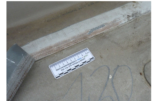
Faulty automatic weld caused by incorrect welding temperature or welding speed.
