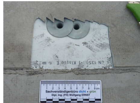
Rupture of the seam welding caused by withdrawal of the welding nozzle.
