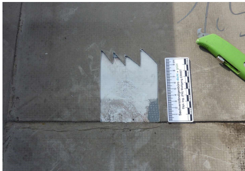
Faulty manual weld at the end of the automatic weld.
