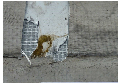
Interrupted automatic weld caused by carbon deposits from the welding nozzle.
